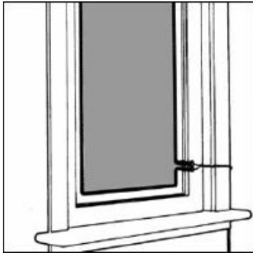
Figure 2 A type of perimeter alarm will activate when the window is broken. When that happens, the foil tape tears, which breaks a circuit and sounds an alarm
