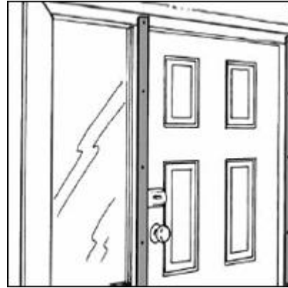
Figure 5 Use long screws to install metal brace on frame of door with sidelights.
