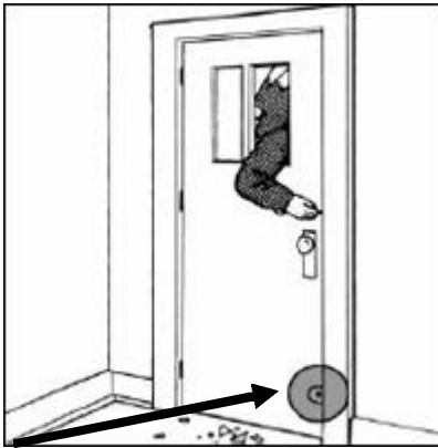
Figure 13 Breaking the glass will not help a burglar if the auxiliary lock is out of reach.
