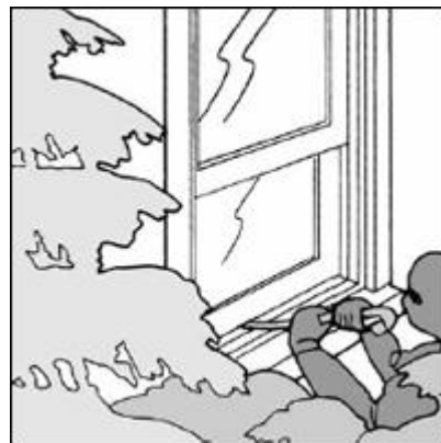
Figure 2 All windows within 2 m (6 1/2 ft) of ground level should be burglar resistant. Secure windows that are easily accessed by exterior structures or accessories, such as balconies or canopies.
